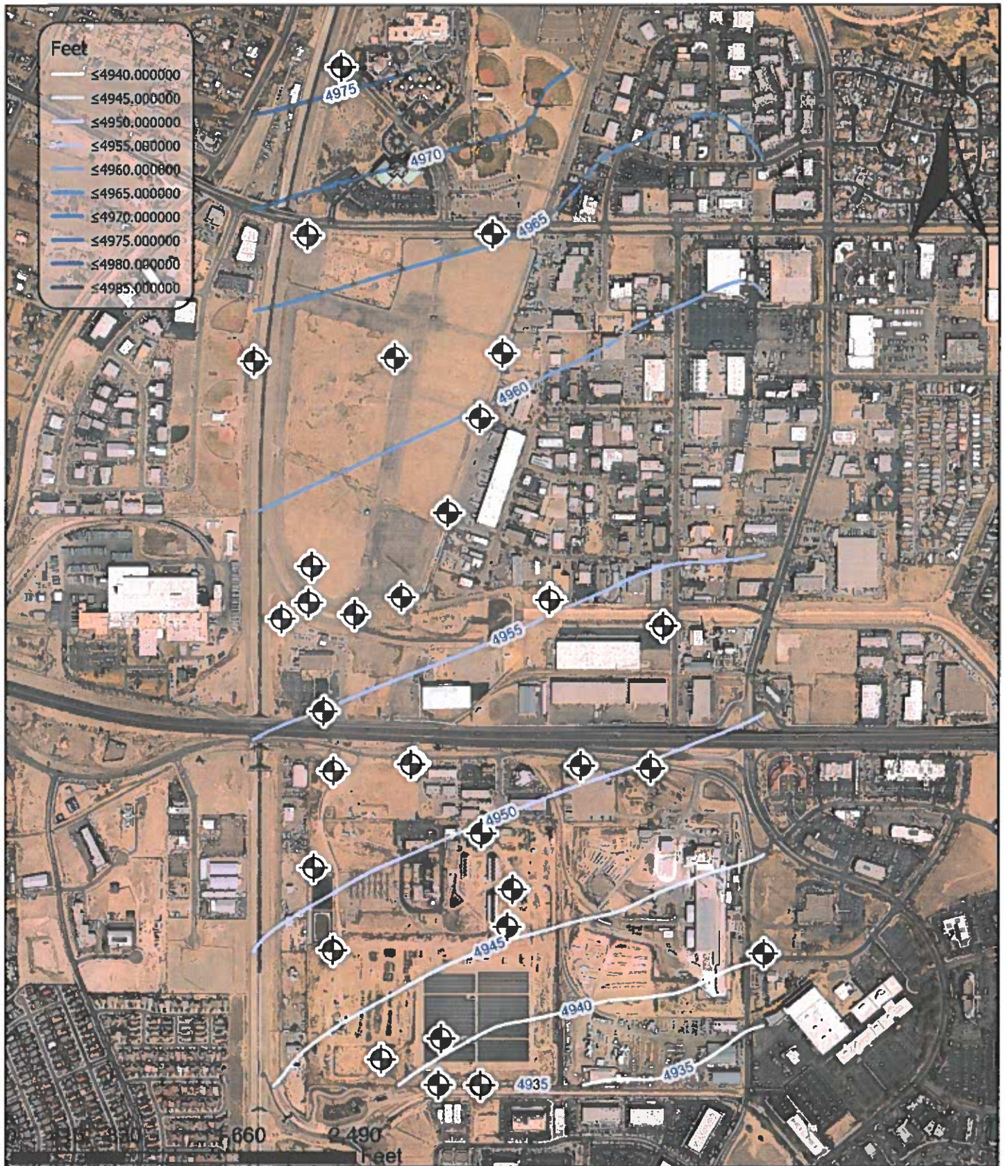
Figure 7 Groundwater Elevation Contours August 2019 H02 2019 Groundwater Monitoring
