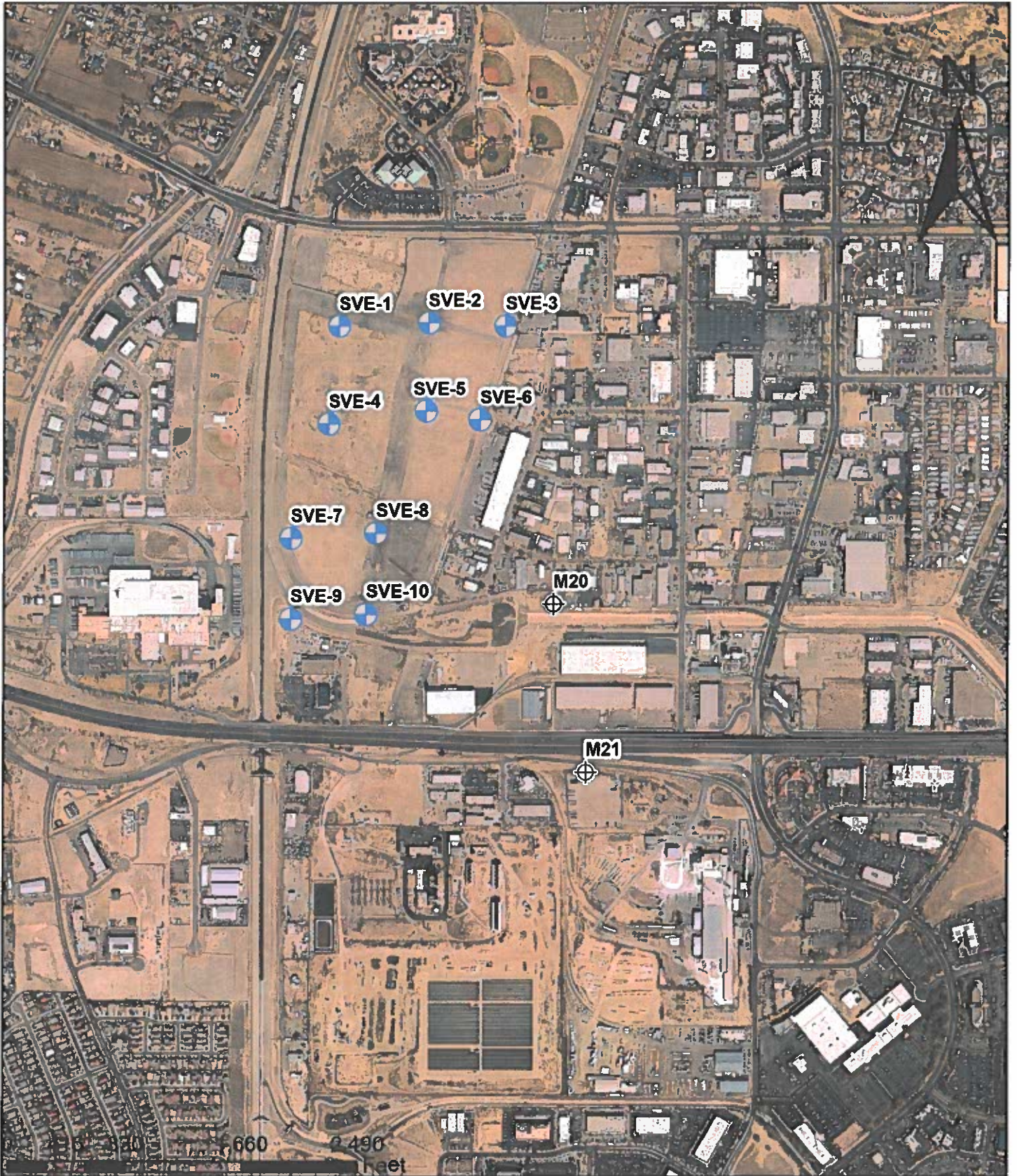
Figure 12 Soil Vapor Sampling Locations
