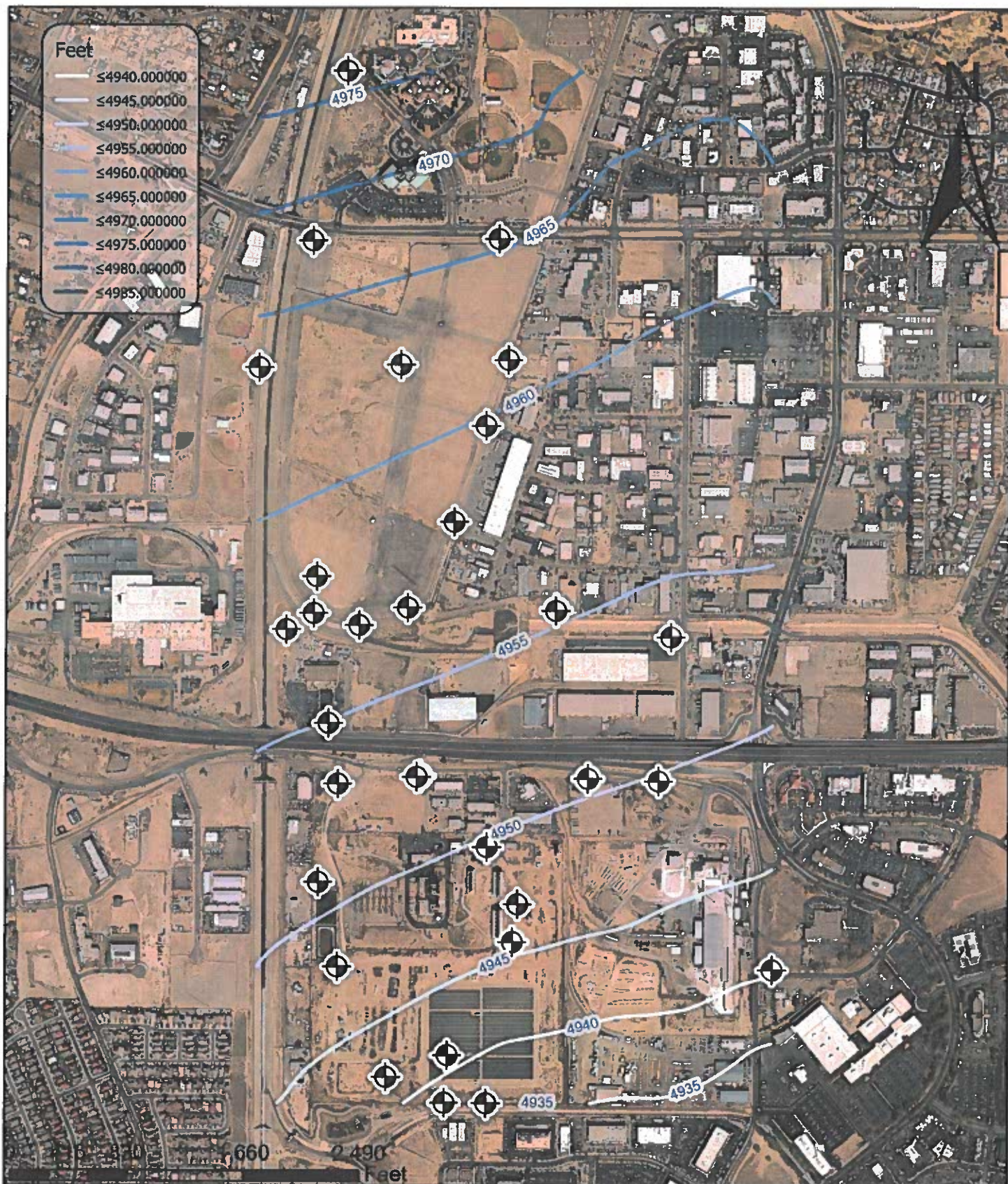
Figure 8 Groundwater Elevation Contours September 2019 H02 2019 Groundwater Monitoring
