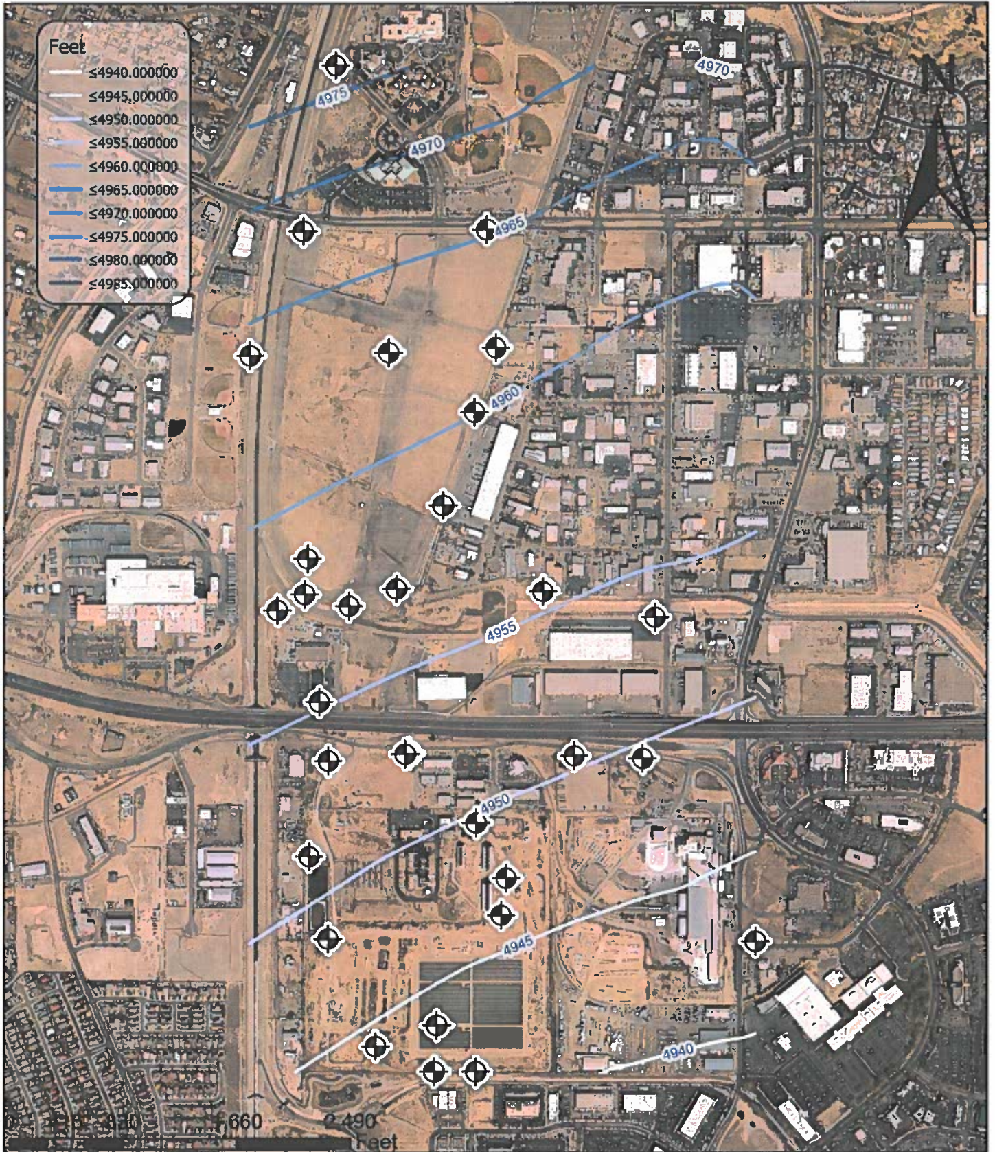
Figure 11 Groundwater Elevation Contours December 2019 H02 2019 Groundwater Monitoring
