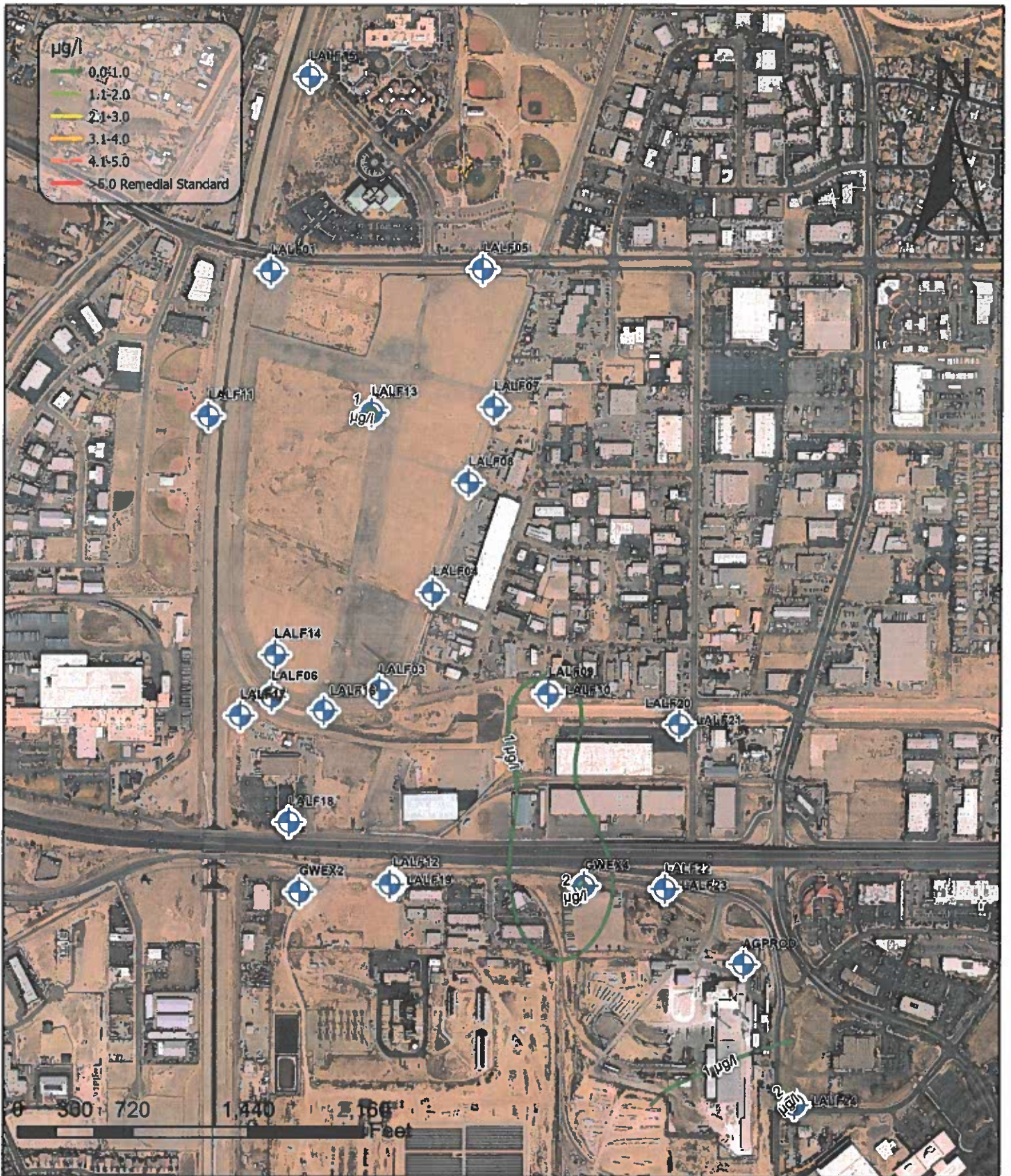
Figure 4 Trichloroethene H02 2019 Groundwater Monitoring
