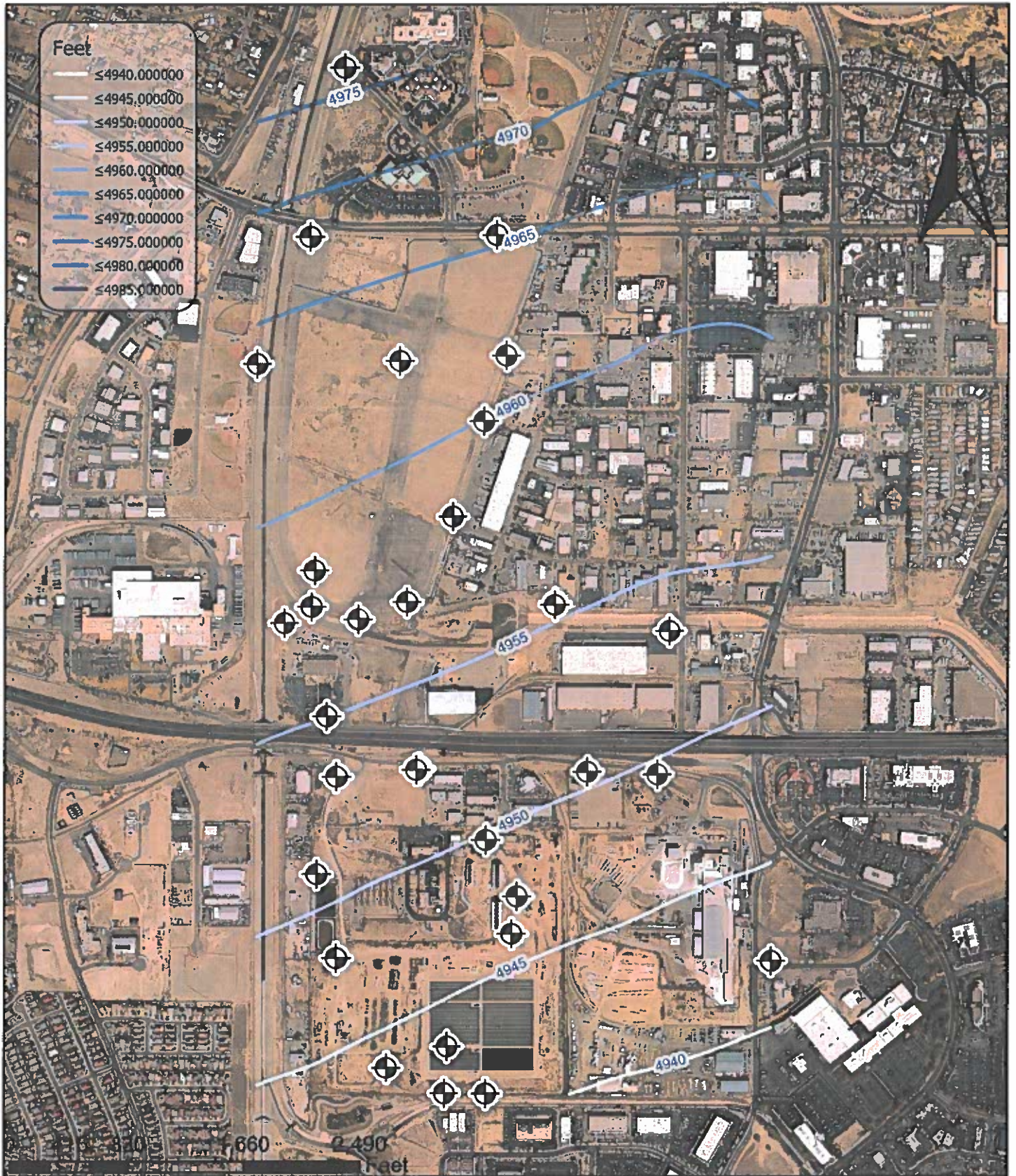
Figure 9 Groundwater Elevation Contours October 2019 H02 2019 Groundwater Monitoring
