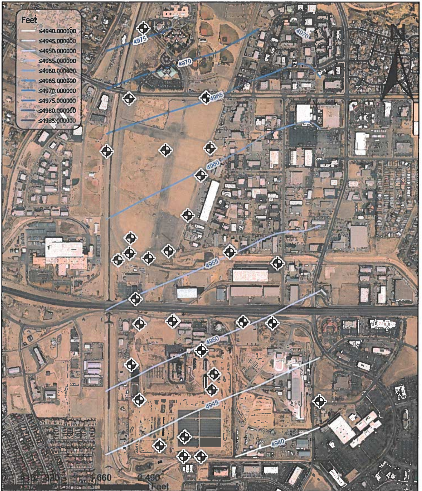
Figure 6 Groundwater Elevation Contours July 2019 H02 2019 Groundwater Monitoring
